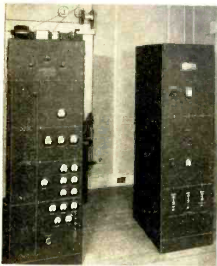
Fig. 4. New automatic recorder and short-wave receiver used by the U. S. Bureau of Standards for recording continuously the signals reflected from the constantly shifting layers of the ionosphere. The unit at the right is the power-supply, that on the left is the first of two sections of the multi-frequency transmitter-receiver system.
